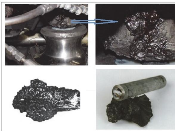
Figure 5. the scabna on the impeder
