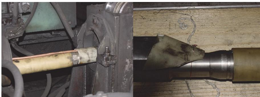
*Figure 7. a) air supply pipe on the impeder bracket, b) "cap" on one side of the impeder*
