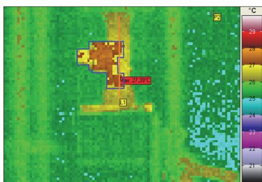
Figure 3. Thermogram of the test sample with an external extensometer
