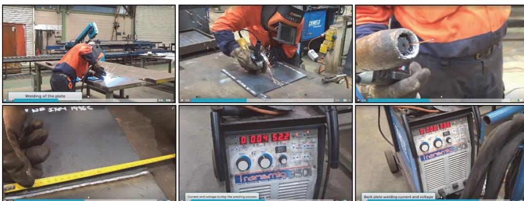
Figure 4. Welding of the test plate
