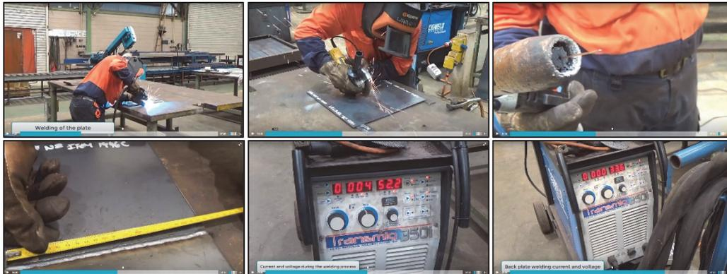
Figure 4. Welding of the test plate
