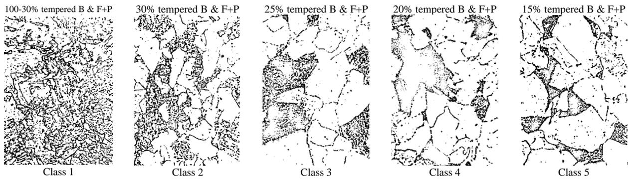
Figure 4. Acceptable classes (1-5) of microstructure of steel 12X1MF
