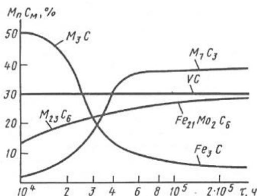
Figure 3. Kinetics of the change in the type and amount of carbide  $M_n C_m$  in the creep process in 12X1MF steel
