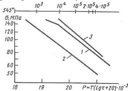
Figure 6. Diagram of creep rupture strength for steel 12X1MF
