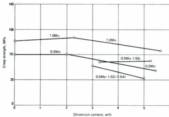
Figure 1. Effects of Cr on the creep strength (stress to produce a minimum creep rate of 0.0001% per hour) of several steels containing small amounts of Mo, Si, Al at 540 °C
