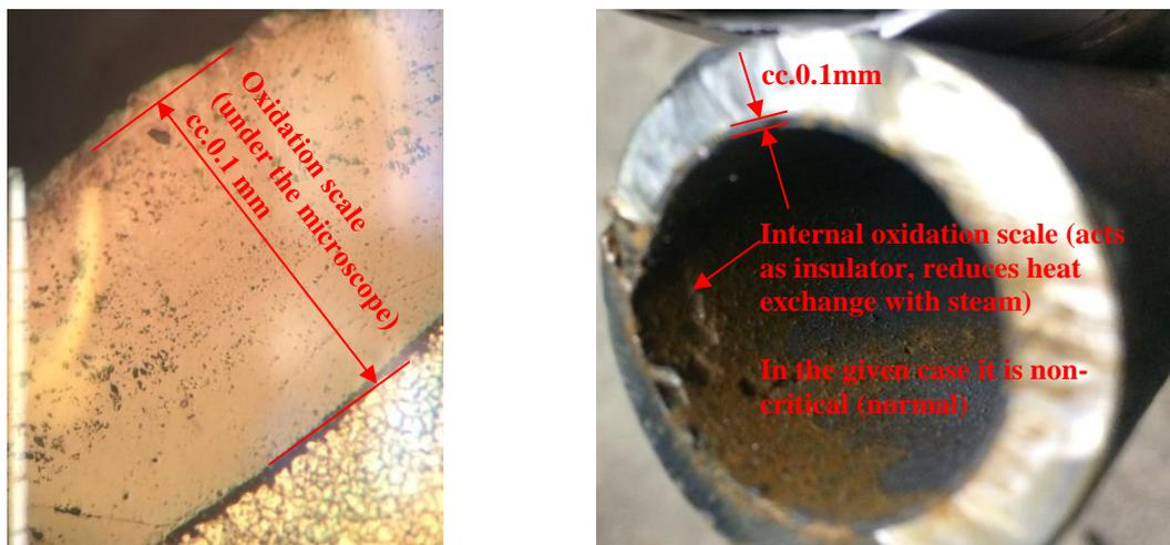
Figure 12. Oxide scale (non critical thickness)
