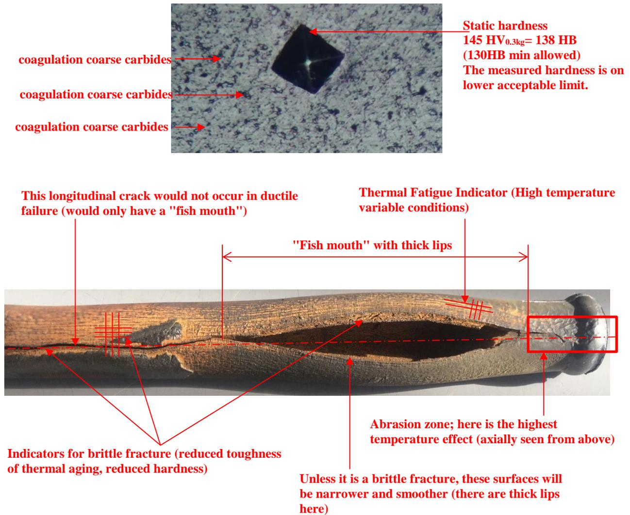
Figure 11. Micro-hardness and visual inspection for creep indicators
