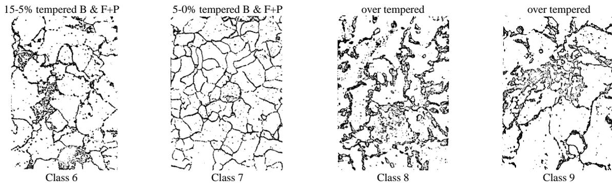
Figure 5. Un-acceptable classes (6-9) of microstructure of steel 12X1MF
