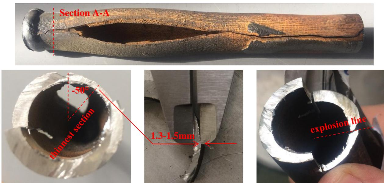
Figure 10. Measurement inspection of exploded segment
