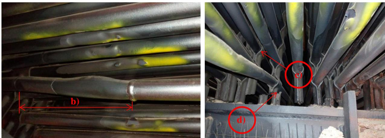
Figure 9. Location and restrains of failure tube segment
