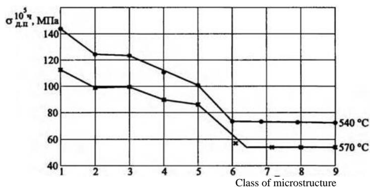
Figure 8. The long-term strength of the metal pipe made of steel 12X1MF, depending on the point of the structure on a scale TU 14-3-460-75 [6]
