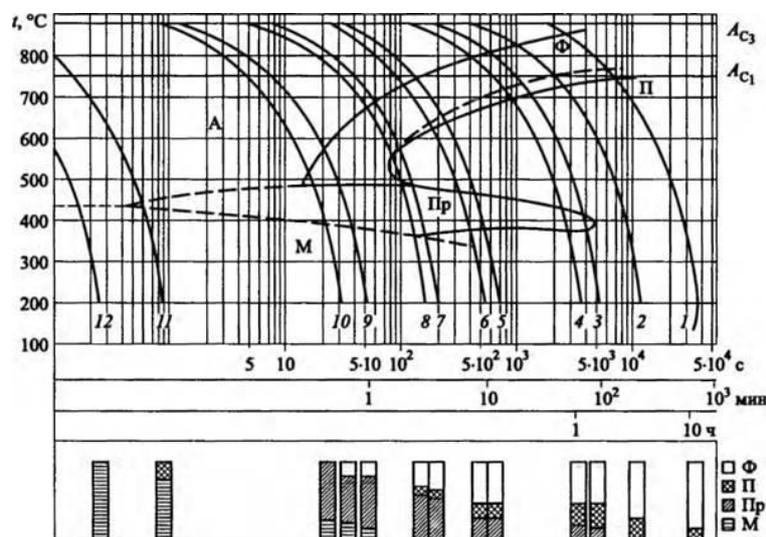
Figure 7. Thermokinetic diagram of 12X1MF steel at a cooling rate, °C/min: 1-1; 2-3; 3-6; 4-10; 5-55; 6-70; 7-185; 8-230; 9-800; 10-1660; 11-cooling in oil; 12-cooling in water; A-austenite; F-ferrite; P-pearlite; Pr-an intermediate phase; M-martensite
