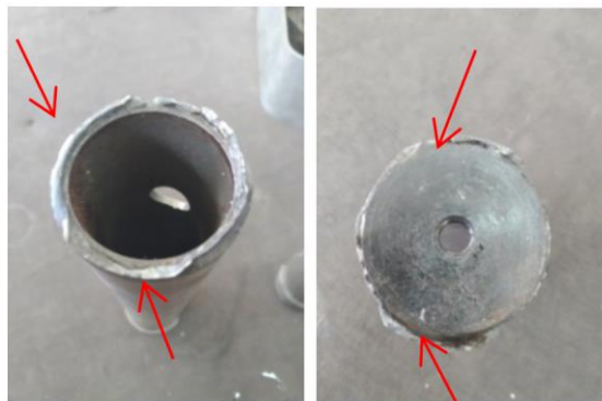
Figure 4. Fracture of the pulling pipe as result of the tensile testing
