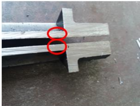
Figure 3. Lack of penetration
