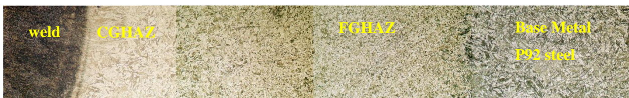
Figure 11. Microstructure of the welded joint
