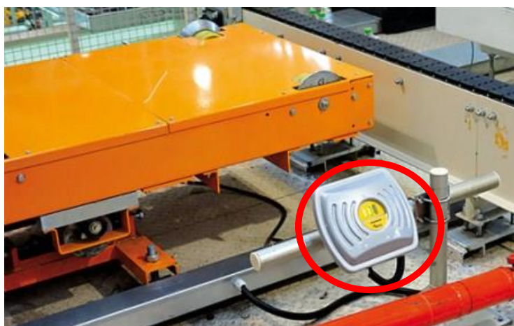
Figure 4. RFID-read/write head for transmission of data from the RFID transponder on the car body 2
