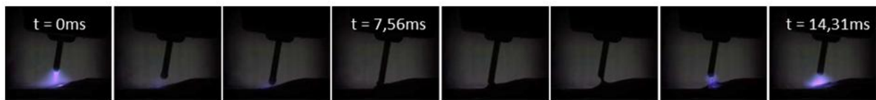
Figure 3. Method of droplet detachment CMT process
