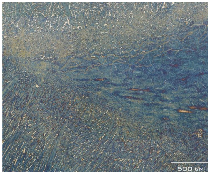
Fig. 3. Weld microstructure formed with a high heat input, visible are radially oriented dendrites and severe grain growth (etched with 7% \text{Na}_2\text{S}_2\text{O}_5 ).
