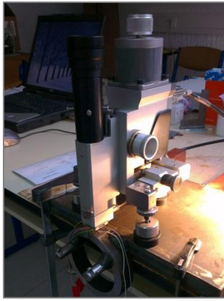
Figure 5. Measuring residual stresses using IHDM: a) positioning the specimen, b) positioning and preparing the strain gauge rosette, c) positioning measuring device above the strain gauge rosette, d) centering the measuring device within the strain gauge rosette, e) performing the measure, f) measuring the hole dimensions after the process of measurement
