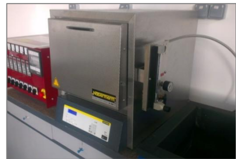
Figure 4. Stress relieving heat treatment: a) stress relieving diagram, b) furnace Nabertherm B180
