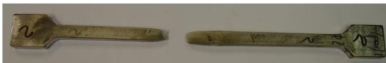
Figure 3: Tensile specimens after testing.
