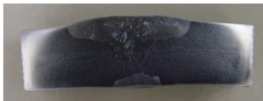
*Figure 2: Macro metallographic sample of the weld joint on 316 L stainless steel*
