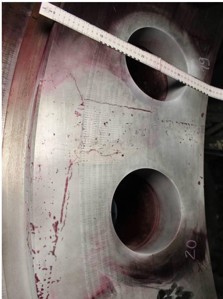
Figure 5. Cracks in the area of the repair weld (between openings for bolts nr. 19 and 20)
