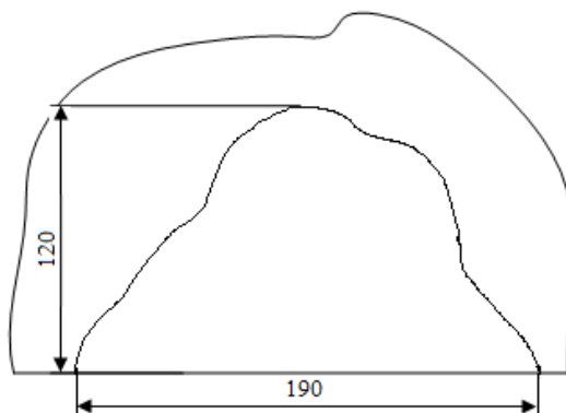
Figure 10. Appearance of the groove at the location where the deepest crack was detected
