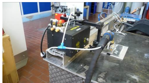
Figure 6. Supply of shielding gas and point of measurement
