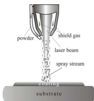
Figure 5. Scheme of laser cladding
