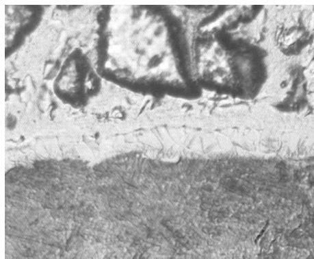
Figure 6. Microstructure of NiCrBSi+WC coating - 42CrMo4 steel substrate, 450:1, etching: nital, light microscope [42]
