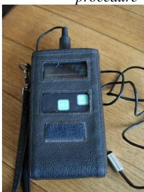
Figure 5. Electromagnetic indicator of surface cracks EMIT 1
