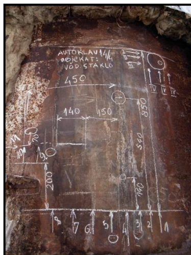
Figure 2. Controlled area of the autoclave with the scheme of the recording routes and the geometry position of cracks
