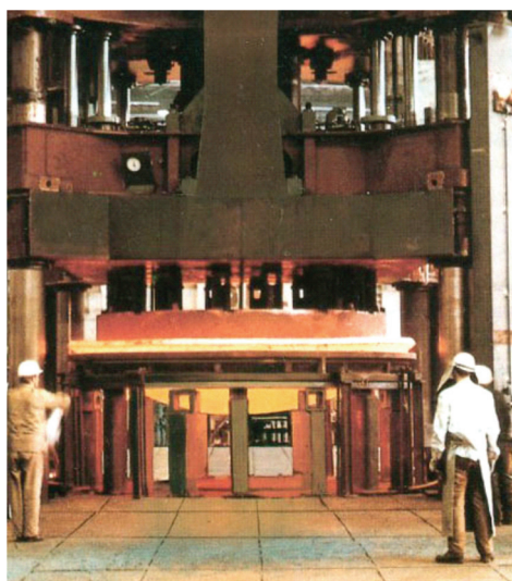
Figure 6: Forming of heated metal plate which is later used as a spherical tank segment
