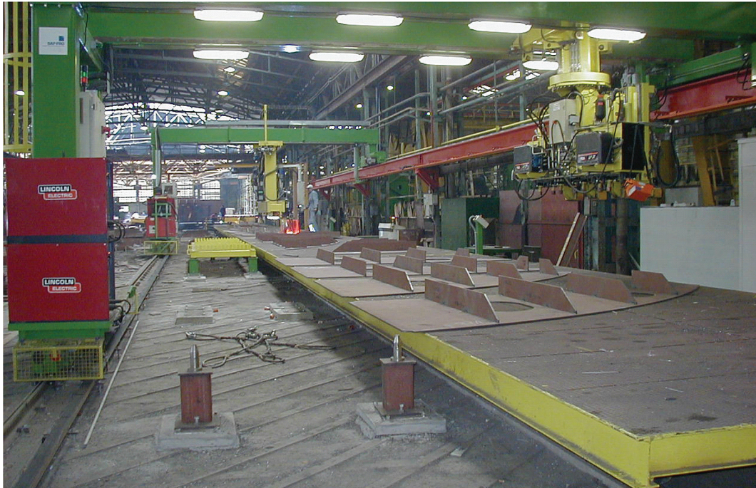
Figure 1: Automated welding line
