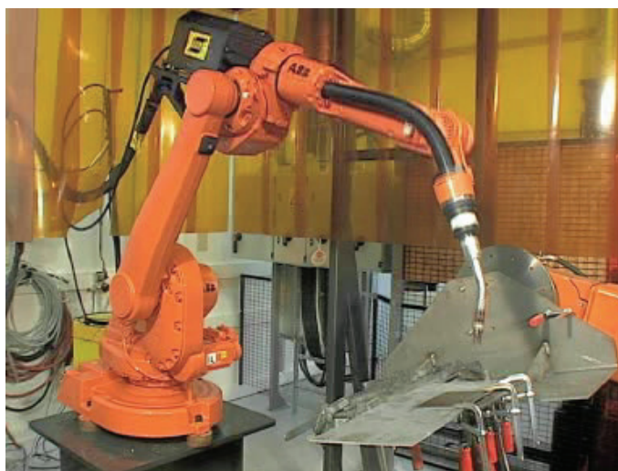
Figure 3. Hollow wrist robot air cooled (Source: ABB)
