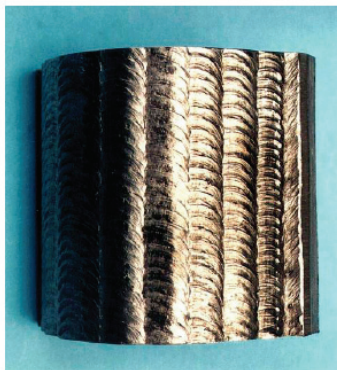
Pipe dimensions: \varnothing 57 \times 6 \text{ mm} Base material: 16 Mo 3
