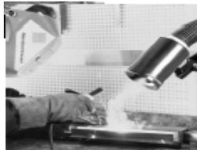
Welding fume extraction with nozzles
