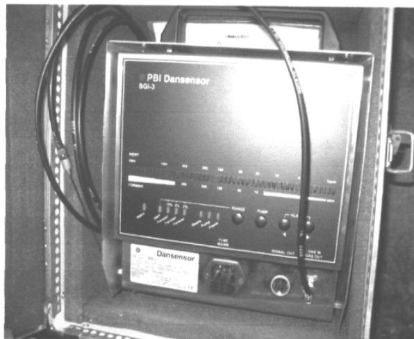
Slika 6: OKSIMETER, tip PBI DANSENON, SG-3
