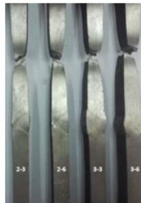
**Figure 3.** Tensile test specimens after testing
