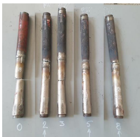
Fig 4. Tensile tested technological probes
