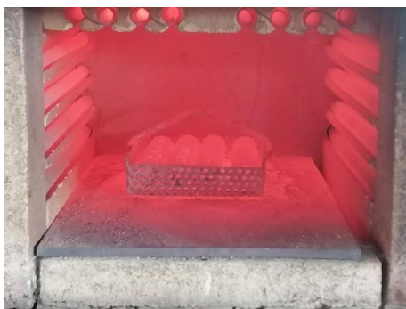
Fig 2. PWHT of steel P91 for 2h
