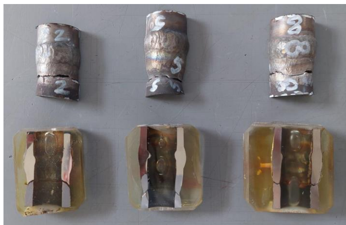
Fig 6. Fracture in HAZ of P91 as result of overheating during buttering with Thermanit Nicro 82
