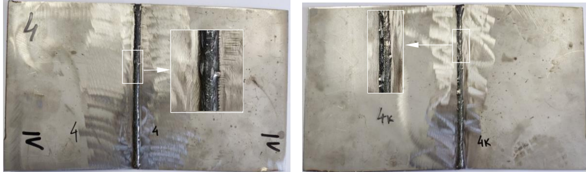
Figure 4. The appearance of the welded joint (face and root)
