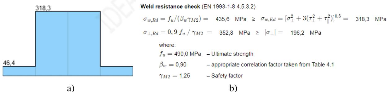
**Figure 4.** a) Equivalent stress distribution in critical weld b) Analytical calculation of critical weld
