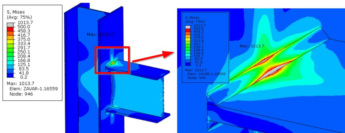
**Figure 7.** Equivalent stress distribution
