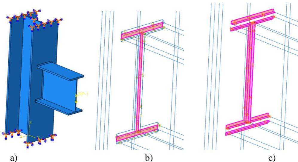
**Figure 6.** a) Encastre BC and concentrated force of 70kN, b) Surface to surface contact interaction, c) Tie constraint between weld and beam
