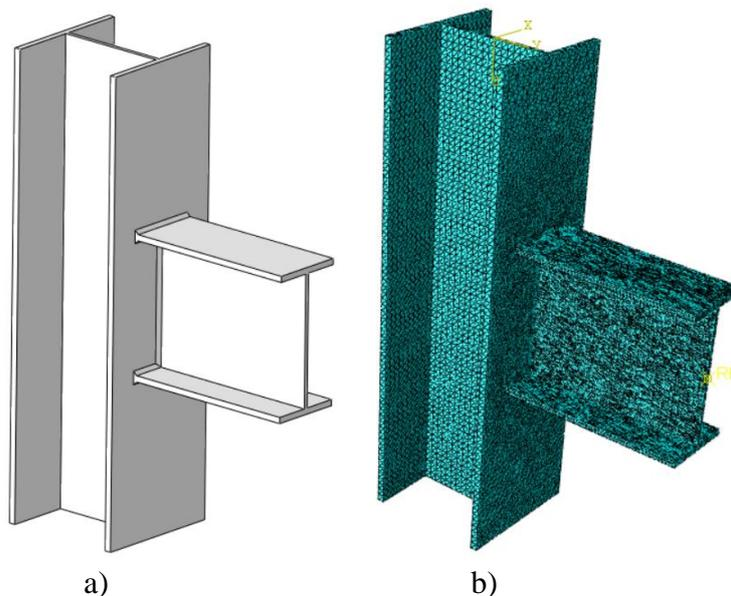
**Figure 5.** a) 3D model without too many details b) 3D model meshed with 10-node quadratic tetrahedron finite elements
