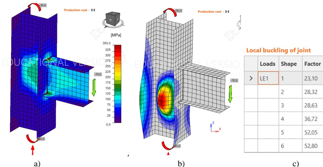
**Figure 3.** a) Equivalent stress distribution in plates and welds, b) First buckling mode of joint, c) Buckling modes and eigenvalues
