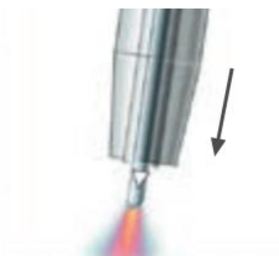
Figure 1 Start of the arcing period [3]
