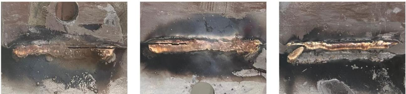
**Figure 3.** Tensile test of the hot-dip galvanized specimens with crack in the diffusion zone. Pulse (left), PMC (middle) & Short-Arc (right)
