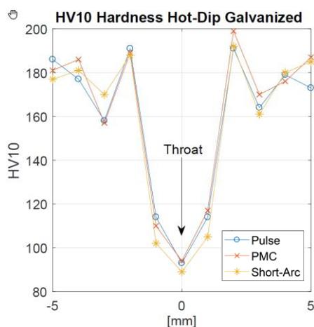
Figure 2. HV10 Hardness of the samples with the throat in the middle of the samples
