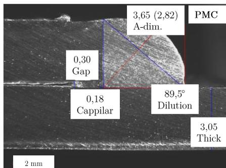
**Figure 4.** Macroscopic evaluation of the PMC brazing with the A-dimension of 3.65 mm and the effective A-dimension of 2.82 mm
