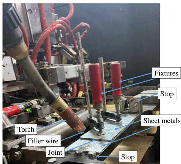
**Figure 1.** Experimental setup at the Reis robot cell
