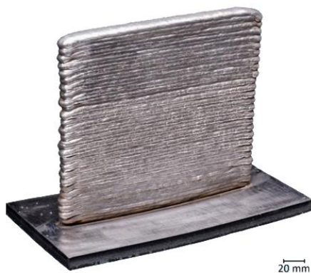
Figure 3. CMT multilayer component made in Inoxline protective atmosphere
