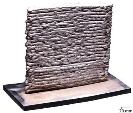
Figure 4. CMT multilayer component made in Argon protective atmosphere
