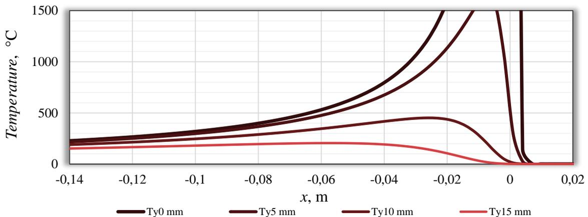
**Figure 3.1.** Temperature field  $q = f(x,y)$  with parametric value  $y$  for  $z = 0$  mm
