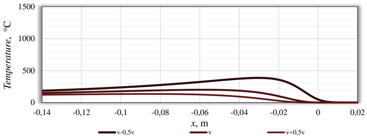
**Figure 3.6.** Temperature field  $q = f(x, y)$  with parametric value  $v$  for  $z = 2$  mm and  $y = 15$  mm
