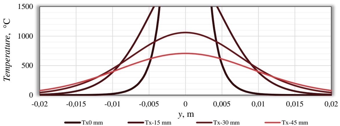
**Figure 3.3.** Temperature field  $q = f(x,y)$  with parametric value  $x$  for  $z = 0$  mm
