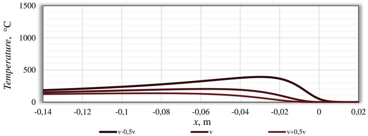
**Figure 3.5.** Temperature field  $q = f(x, y)$  with parametric value  $v$  for  $z = 0$  mm and  $y = 15$  mm
