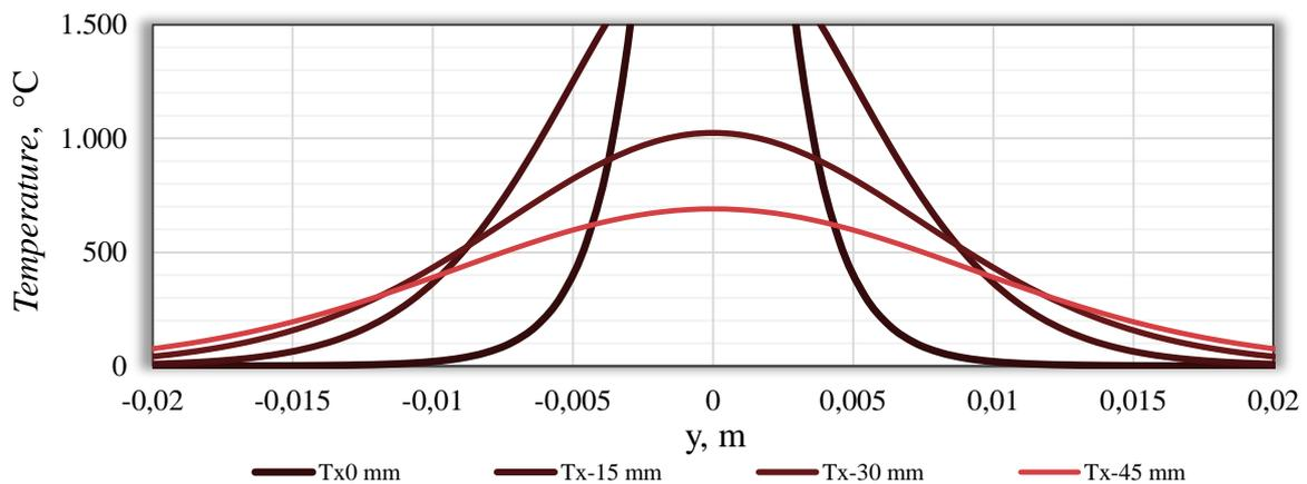
**Figure 3.4.** Temperature field  $q = f(x,y)$  with parametric value  $x$  for  $z = 2$  mm
