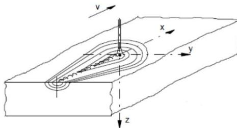
**Figure 2.1.** Moving point source on a thick plate
