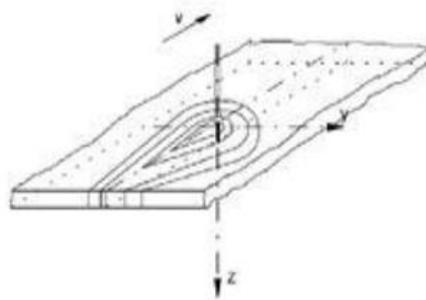
**Figure 2.2.** Moving linear heat source on a thin plate
