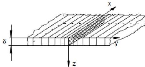
**Figure 2.3.** Instantaneous planar heat source
