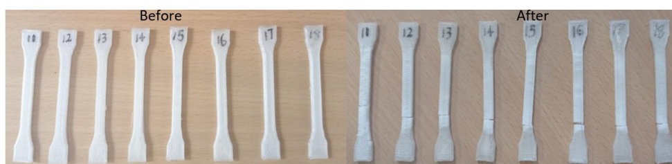
Fig. 6 Specimens before and after tensile testing
