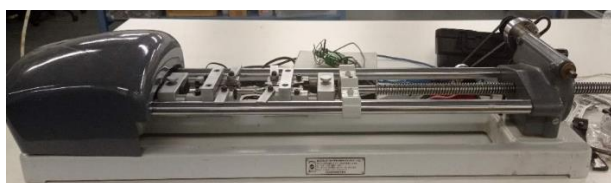
Fig. 4 Electronic tensometer, Model PC-2000
