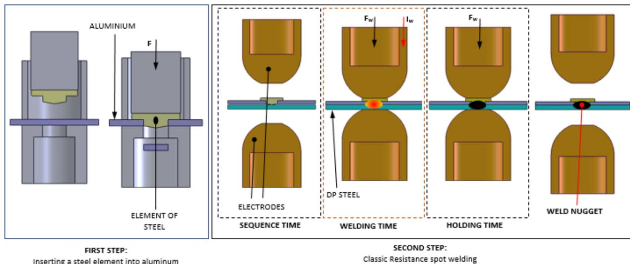
**Figure 1.** Process of Resistance element welding (REW) [7]
