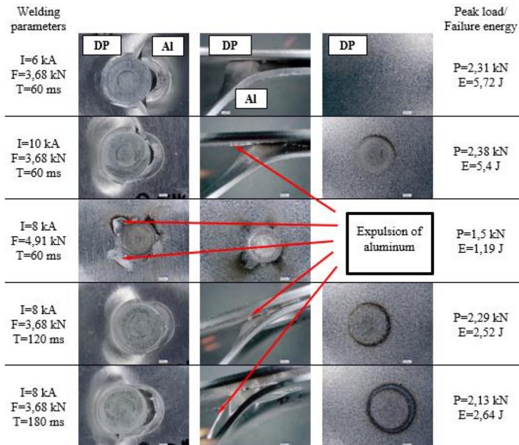
Figure 2. The results of tensile-shear testing
