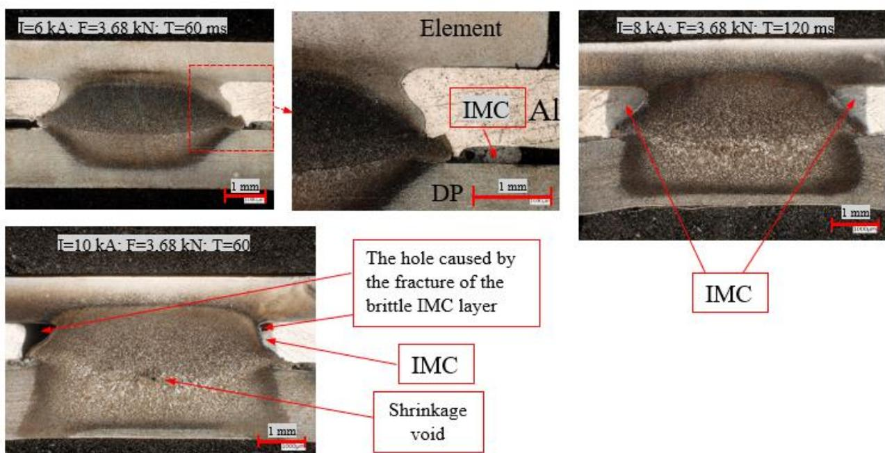
**Figure 3.** The Macrostructure of the REW joint of DP500 steel and aluminum alloy AW 5754
