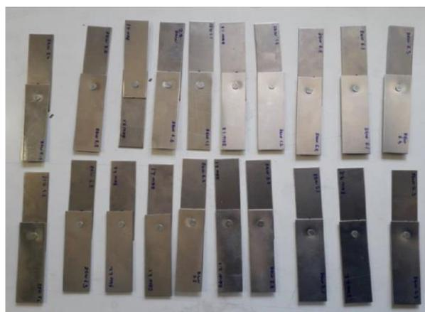
**Figure 1.** Specimens prepared for tensile-shear test
