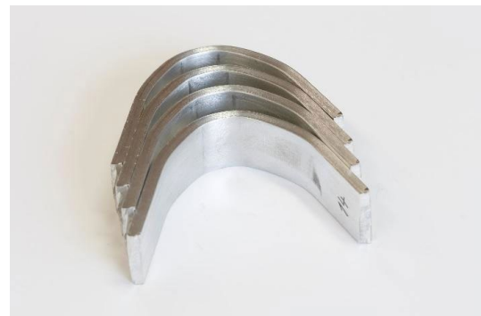
Figure 13. Welded joints after bend test from surface part
