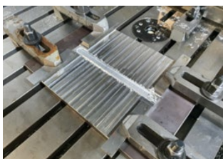
Figure 2. Welding setup and clamping
