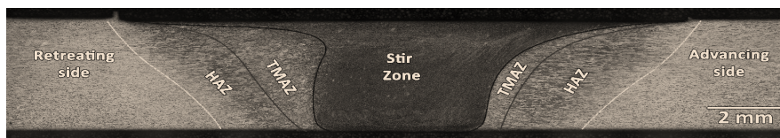
Figure 5. Macrostructure of Sample 14
