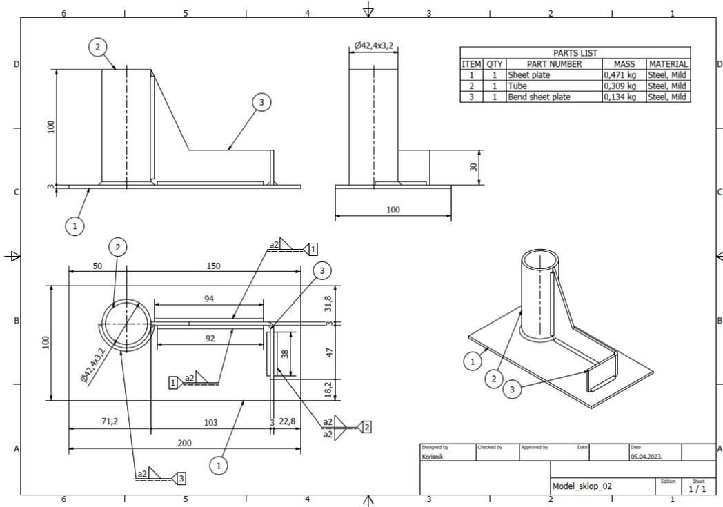
Figure 14. Model drawing with material table
