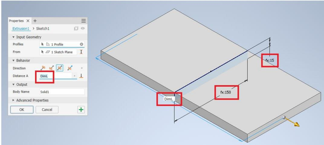
Figure 5. Modeling dialog with parameter for dimensions
