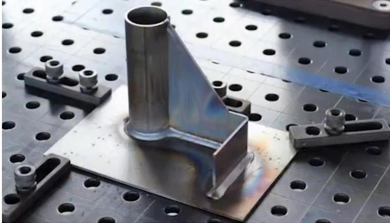
**Figure 19.** Finished product welded by COBOT
