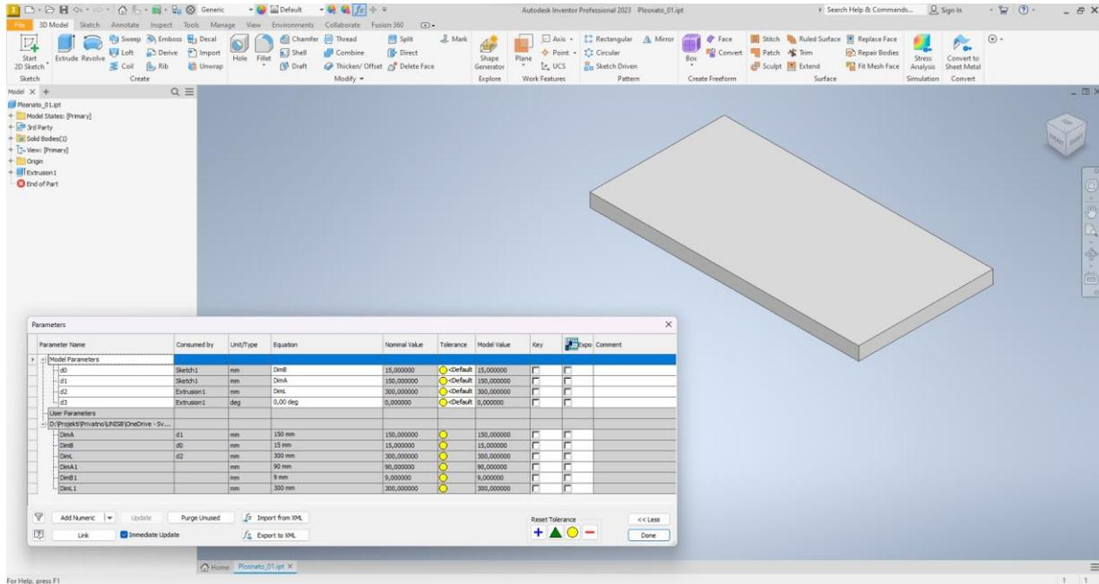
Figure 3. Inventor model with parameters dialog
