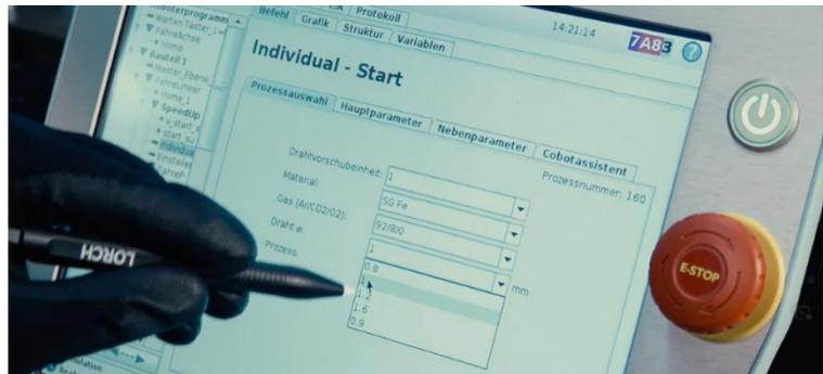
Figure 15. Definition of materials and processes parameters in COBOT software
