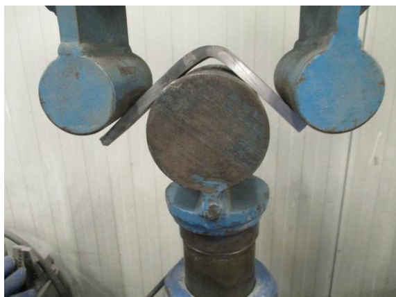
Figure 9. Bend testing of weld root
