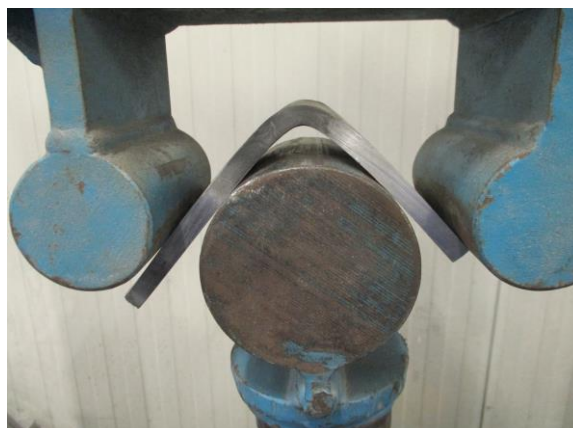
Figure 10. Bend testing of weld face
