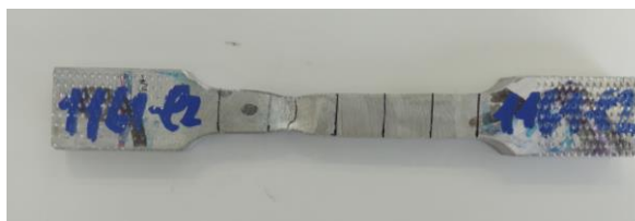
Figure 7. Tensile test fracture specimens
