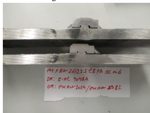
Figure 2. Macro structure butt welded joints with backing strip butt welded joints with backing strip
