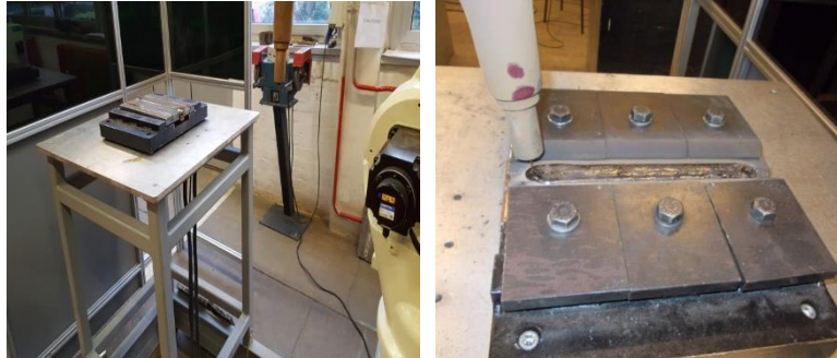
Figure 4: The photo of the weld setup taken immediately after welding [4].
