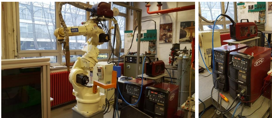
Figure 5: The photo of OTC FD-V20S robot and welding sources M500D used at welding [4]
