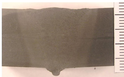
Figure 10: Macrosection of the weld joint
