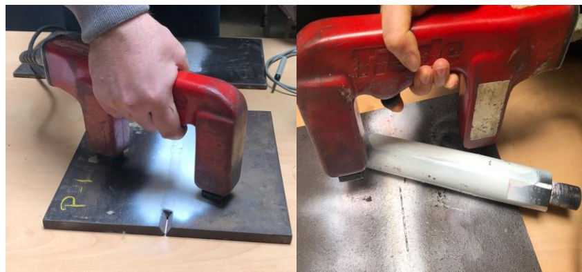
Figure 11. Specimen testing procedure with electromagnetic yoke
