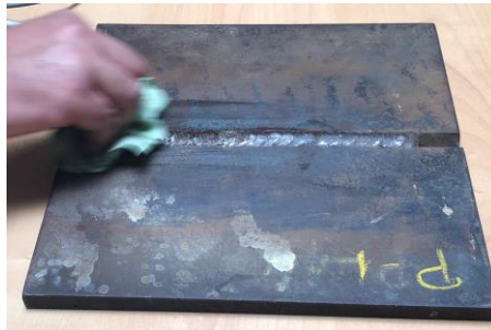
Figure 7. Cleaning the surface of a metal plate with a weld
