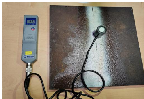
Figure 6. Measurement of workplace illumination with a lux meter
