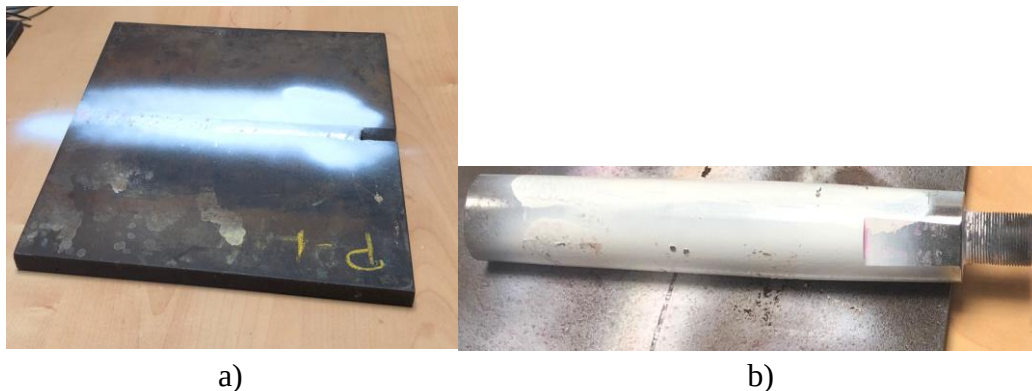
Figure 10. Contrast agent and magnetic particles on test specimens: a) metal plate with weld and b) metal shaft without weld
