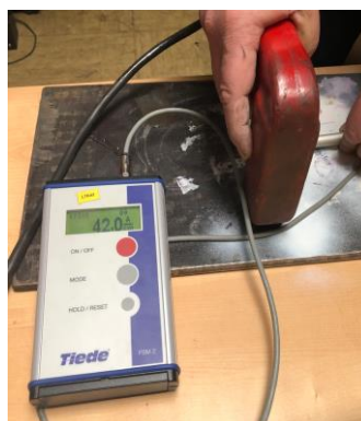
Figure 9. Measurement of magnetic field strength
