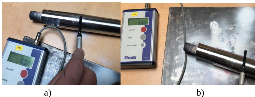
Figure 15. Measurement of the magnetic field strength: a) before demagnetization and b) after demagnetization
