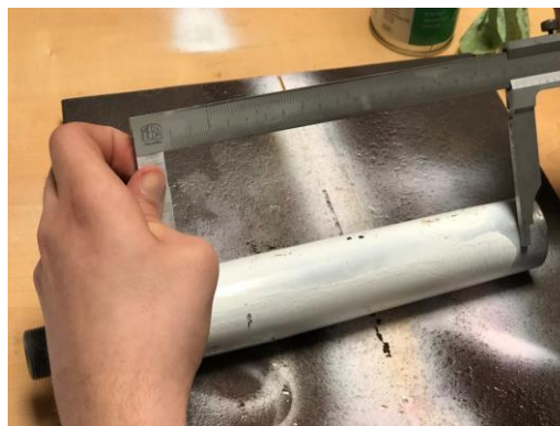
Figure 13. Determination of the position and dimensions of the metal shaft defect
