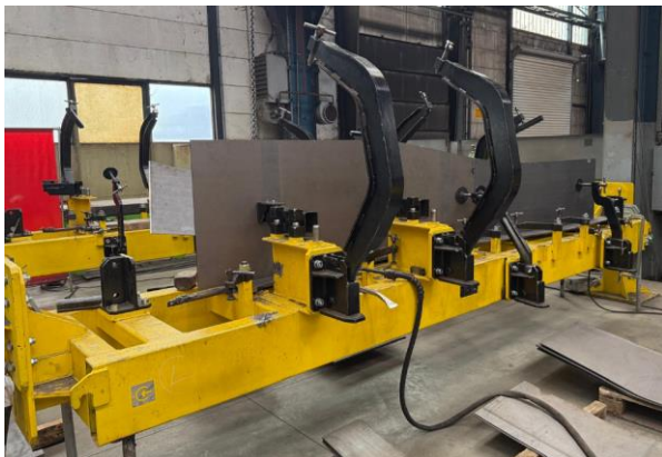
Figure 14. "S" beam fixture
