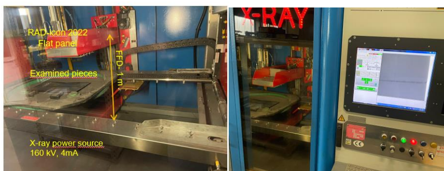
Fig.3 Welding defects capturing system
