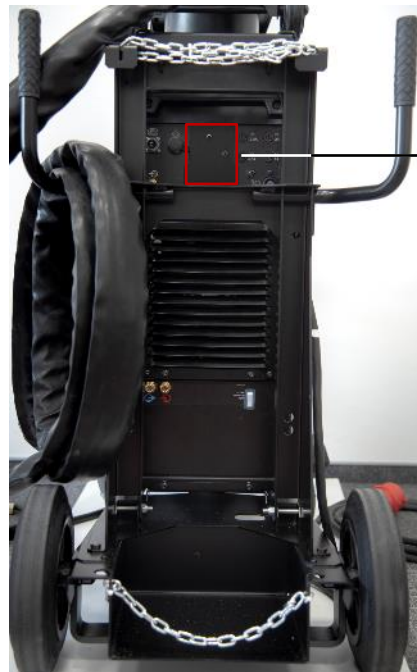
Cable connections on back rear side with optional K14337-1 KIT
