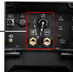
Cable connections on back rear side with optional K14337-1 KIT
