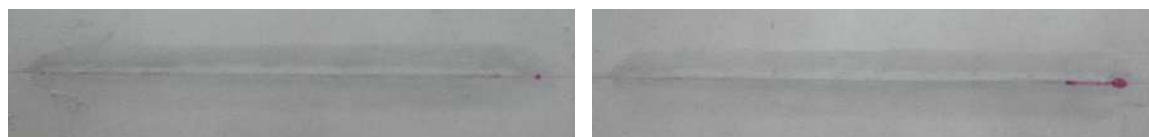
Fig. 5 NDT inspection of weld joints by liquid penetrant
