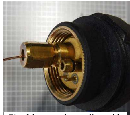
Fig. 8 hose pack coupling with gasket
