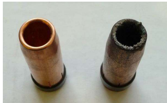
Fig. 9 Gas nozzle with and without spatters
