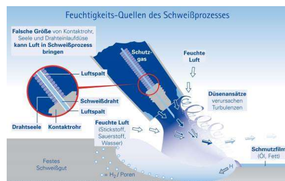
Fig. 10 Torch and its causes of pollution
